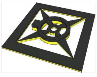
With perfect Z-bottom settings, you will be able to see 'daylight' through the wax after doing a rough cut of the second side of the ring and spigot. At this stage you should inspect the surface of the wax and check that your Y-setback settings were correct.
