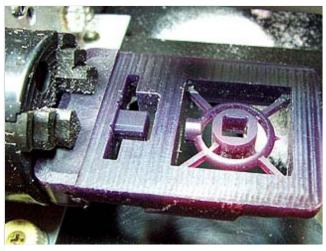
The FlipFlopWax template has the appropriate clearances for tools and shanks where required, counterbores and chamfers around seating/interfacing edges, radii and slopes to allow access, and orientation markings to assist you remounting the ring correctly. Any roughing of the template and spigot can be done with a 1mm / 0.04" ball mill.
