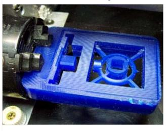
At this stage, all Side-A and Side-B work is complete. Your rotary cutting, or index cutting toolpath should be next in FARM's process list.
