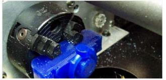
Your machined hub should be a tight fit over the spigot. We recommend the use of a soldering iron to carefully secure the hub and spigot together in a few places, as this kind of join is unlikely to fracture with tool vibrations.
