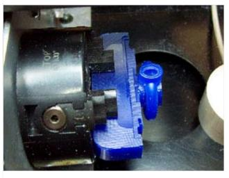
Now you only need to complete a finishing cut on the rotary axis. This pass will neatly remove the protrusions where the outer spokes were used to support the ring.
