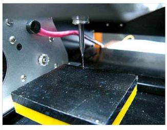
Again, if you have a stock of identical wax blanks, if you are confident about their size and your mounting of them, you may not need to perform this facing operation. We face the block so that the roughing pass is fast and predictable with no gouging.
