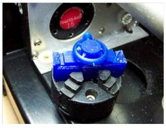
Now all machining is complete, the final ring can be removed by carefully cutting the inner spokes, and leaving the hub behind on the spigot.
