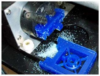
Leaving the wax mounted, with the use of a hot-air knife, a soldering iron, or a small saw, you can now physically separate the crust (including the ring) from the spigot.
