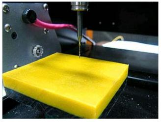
If you know the size and dimensions of your wax, it may not be necessary to face it, but this operation means there is less risk of snapping tools or gouging deeper than the cutter can handle.
