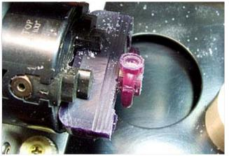
FLOP, the wax hub is a perfect fit onto the spigot, and can now be secured using either a soldering iron or electrothermal 'wax pen' to prevent the tiniest movement. You need not worry about the outer spokes protruding from the ring; these will be machined down in your rotary pass.
